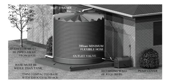
**NOTE:** FAILURE TO PROVIDE A STABLE BASE OR INSTALLING TANK BELOW GROUND LEVEL WILL VOID WARRANTY.
